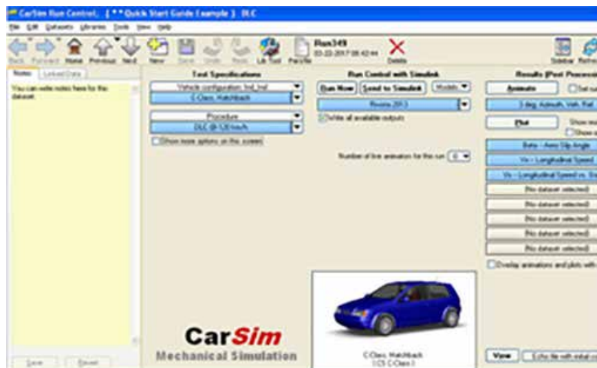
Fig. 8. Panel frontal del software CarSim-Simulink.
